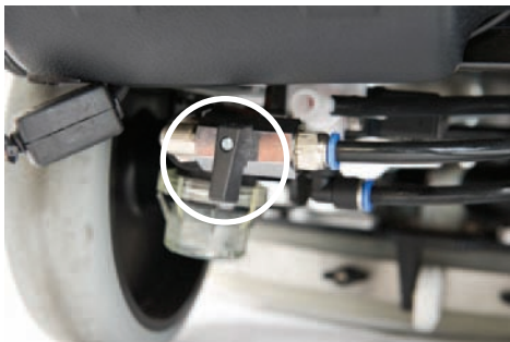
Fig 15 Solution tap fully opened
